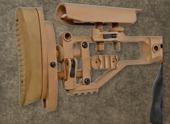
ADJUSTABLE BUTTSTOCK» Tool-free adjustment for length of pull, comb height, and recoil pad height, with locking throw levers to ensure that the settings do not change until the operator wants them to.
