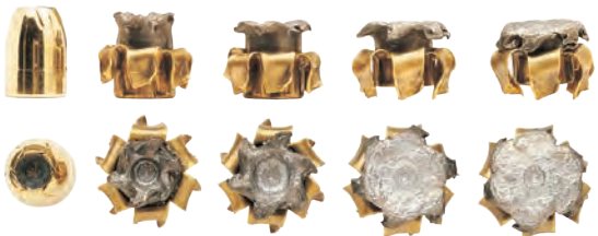
This series of photos shows the totally controlled and extremely uniform expansion of Golden Saber® HPJ bullets.
